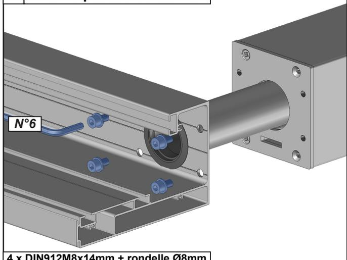
4 x DIN912M8x14mm + rondelle Ø8mm
